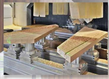
5-axes unit with cardanic 24 kW spindle while drilling horizontal holes.
